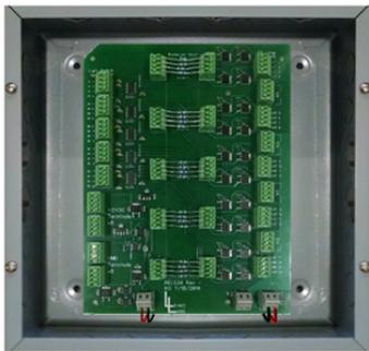
Conturrent takes a different route by having a small control panel, that can be located anywhere, manage an entire low voltage DC system. The panel can be hardwired or even plugged in to a dedicated 15 A line. From there it controls the current going to each lamp circuit providing low voltage DC power.
